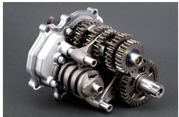
Fig. 11 Cassette type transmission
